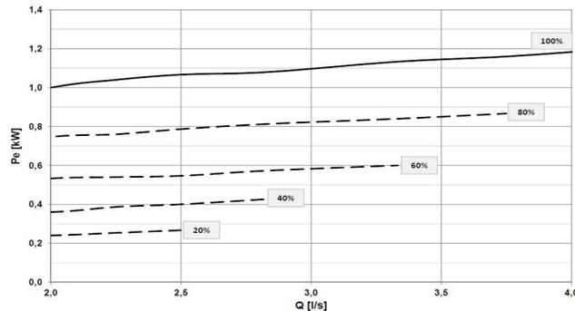
Q = Water flow-rate [l/s] Pe = Electric power consumption [kW]
