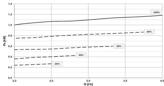
Q = Water flow-rate [l/s] Pe = Electric power consumption [kW]
