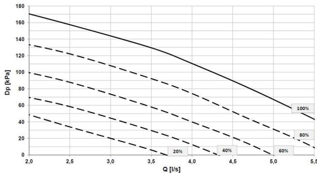
Q = Water flow-rate [l/s] DP = Pressure head, available to the unit fittings [kPa]
