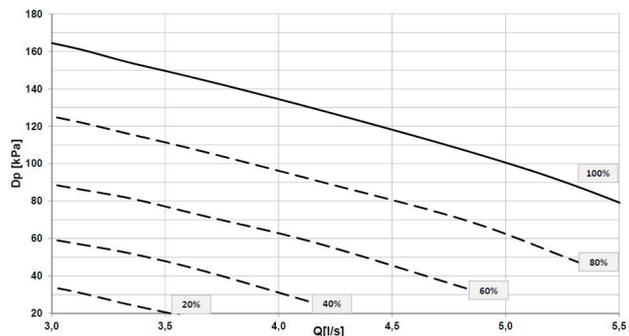
Q = Water flow-rate [l/s] DP = Pressure head, available to the unit fittings [kPa]
