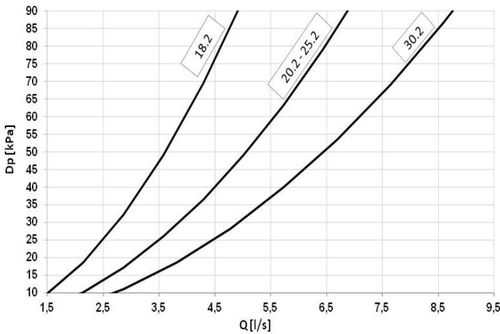
Pressure drop water side are calculated considering a mean water temperature of 7°C
